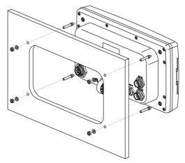
Figure 2.2a - Example of Flush installation CPF300i
